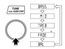
\*This vehicle is not equipped with rear speakers. Adjust the audio control knob, so the level is even.
