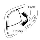
To lock any door with the door-lock button from the outside, push its doorlock button and close the door.
