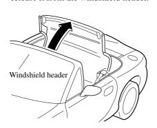
7. Fold back the front and carefully lower it to the storage area, then put the latches in the locked position.
