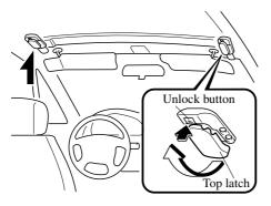
6. Lift up on the front section of the top to release it from the windshield header.
