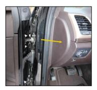
2. With your fingers, pull the weatherstrip away from the door <u>only</u> in the area of this trim panel. The weatherstrip will release when you pull it straight out <u>toward the front of the dashboard</u>.
