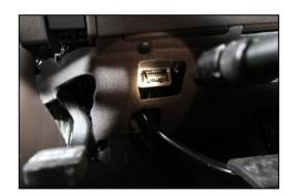
12. From the opening on the left side of the dash, fish the end of the zip-tie out of OBD2 port opening below the dash, following the light from the flashlight.
