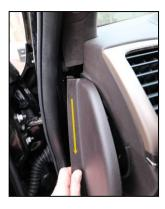
7. Place your fingers behind the headlight control panel and push the lower end out ('1' in photo) while pressing the spring clip upwards under the center bottom of the rear of headlight control panel enclosure.
