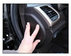
21. Press the loose weatherstrip firmly and evenly back into place. Make sure it is fully seated and smooth with no lumps.
