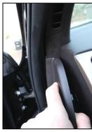
19. Carefully align all 5 tabs and clips with their respective openings on the side of the dashboard.
