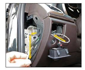
11. Point a flashlight below the OBD2 diagnostic connector <u>under the dashboard</u>, which is just to the right of the parking brake.
