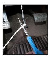
14. Plug the small black connector from the *Smart*StopStart module and the mating connector on the wire from step 12 together until they click. They only fit together in one orientation as shown.
