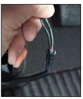
15. Push the wire out of sight in the cavity beside the OBD2 connector and plug the *Smart*StopStart module into the OBD2 port.
