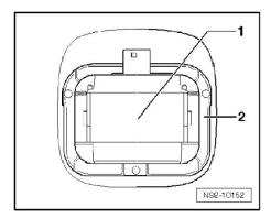
Using a screwdriver, pry Rain Sensor - G213- or Rain/Light Recognition Sensor - G397- -1- from bracket -2-.
