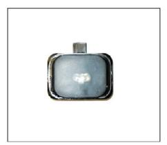
• Identify rain sensor 1K0955559R/T (there is only one set of diodes in the center of the part that contacts the windshield).
