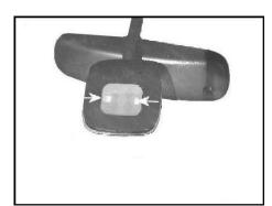
• Install improved rain sensor Part No: 1K0955559AB.
