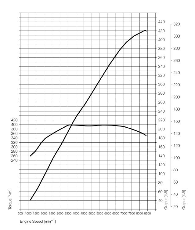
Output and Torque Diagram.
