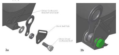
2. Figure 2a shows sequence of hardware fitment. Figure 2b illustrates final fitment on driver outboard seat bracket.
