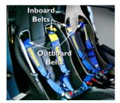
Note: Please read Schroth guidelines for installing ASM shoulder harness. It is critical that the ASM belt is on the inboard shoulder. The ASM belt has a bright yellow tag sewn in (as shown in the image). The Sector111 Harness Kit is designed to help you install the <u>lap belts</u> on ANY Schroth Profi-II belt system (ASM, HANS, etc).
