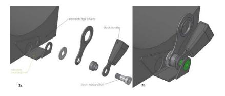
2. Figure 2a shows sequence of hardware fitment. Figure 2b illustrates final fitment on inboard seat bracket.
