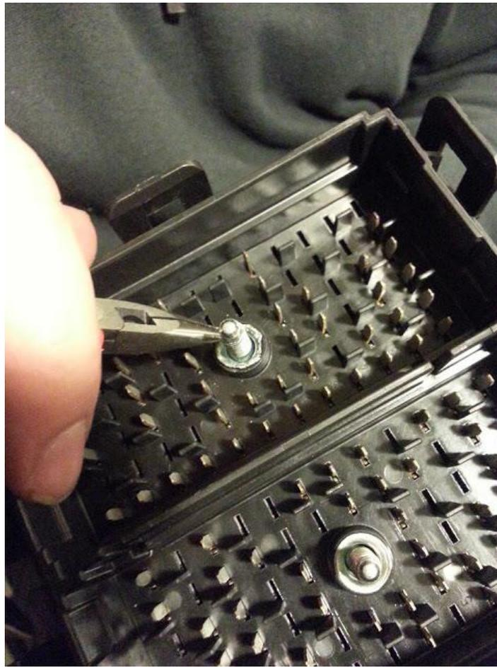
3. When un-swaged enough, knock the bolts through the box so that it can be disassembled. I messed up the bolts so badly (bad needle nose pliers) during the un-swedging that I decided to cut the metal sleeves surrounding the bolts (see picture) so that they don't interfere. The sleeves are not needed as their only purpose is to keep you from opening the fusebox. When the box is in the car, it is held in place by the four bolts and the four block modules.
