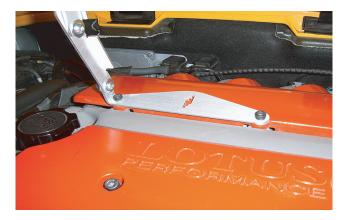
3) Remove stock 10mm nuts holding trunk locking mechanism on the underside of the engine lid (image 3A). Release stock lid prop and lift engine lid near to its top limit (close to the roll bar cover). Fit top of LIDbone on trunk lid studs and secure using stock 10mm nuts (image 3B). We recommend using medium or full strength thread locker to secure these nuts.
