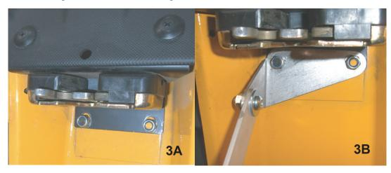
4) The LIDbone will automatically lock in place when trunk lid is opened. To close the trunk lid, hold lid with one hand, and push LID bone towards passenger compartment with other hand until locking mechanism releases. If motion is too stiff or too loose, you can adjust allen bolts and nuts on hinges accordingly until motion is smooth. **Make sure LIDbone is installed as shown in image below.** Enjoy!
