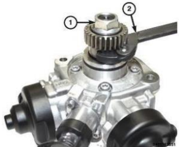
Figure 16 - Spanner Wrench and Drive Gear on the HPFP
