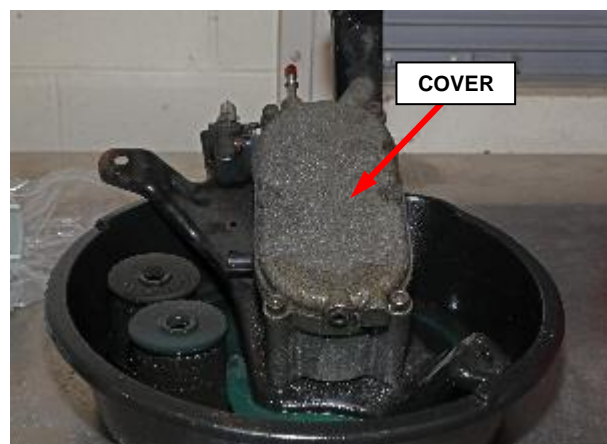
Figure 27 - Remove Fuel Filter/Water Separator Cover
