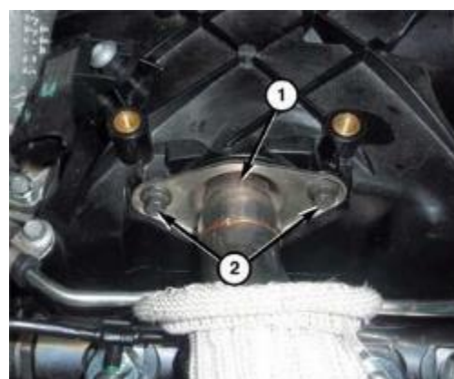
Figure 45 - Upper EGR Tube Bolts at Intake
