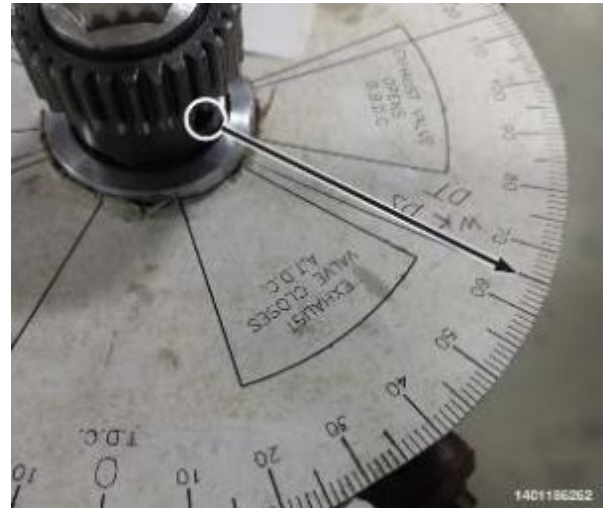
Figure 15 - Installing a Printed Paper Degree Wheel from the Internet
