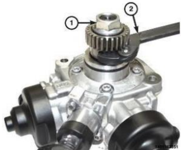
Figure 53 - Spanner Wrench and Drive Gear on the HPFP
