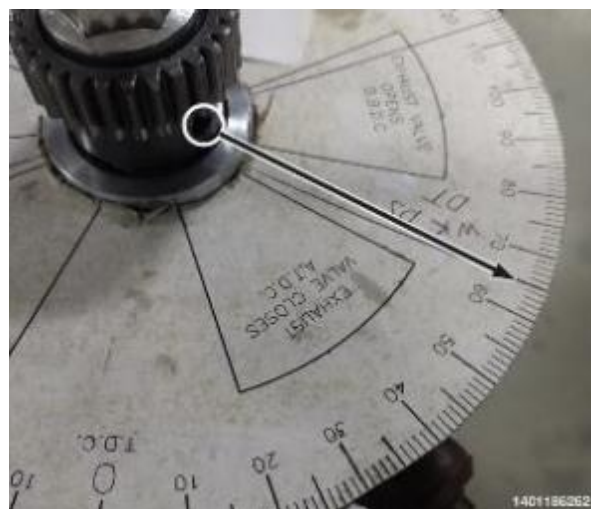
Figure 51 - Installing a Printed Paper Degree Wheel from the Internet
