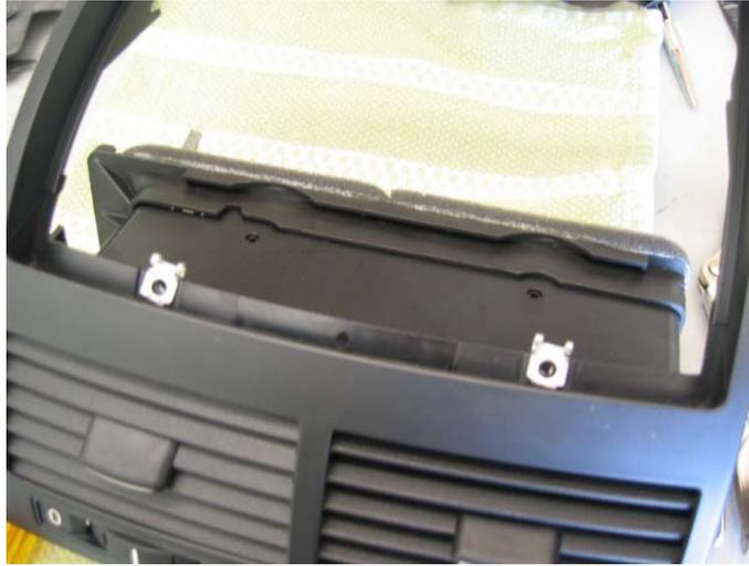
13. Insert 2 screws through front of bin and into speednuts. Tighten with screwdriver. Be sure to press bin tightly onto assembly and screw down firmly.
