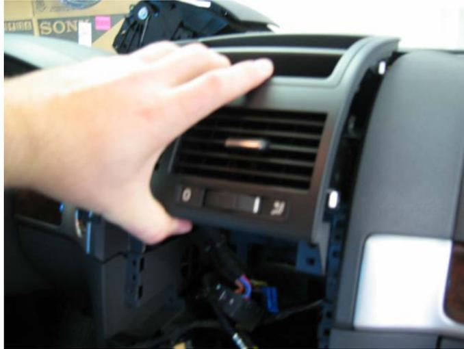
8. Unplug small electrical connector from underside of assembly using your thumb. It's a small tab.
