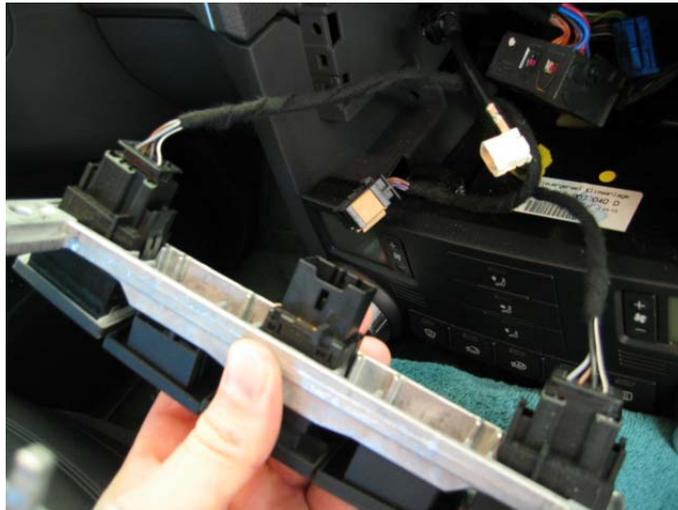
7. Firmly pull vent and storage assembly straight out toward rear of vehicle. The entire assembly will pop out.
