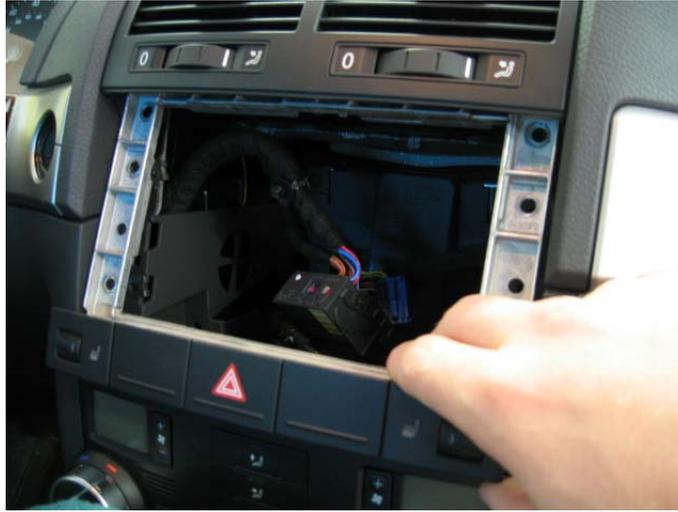
6. Unplug hazard and seat heater controls by pressing on tabs on the rear of the controls. Place bracket aside.
