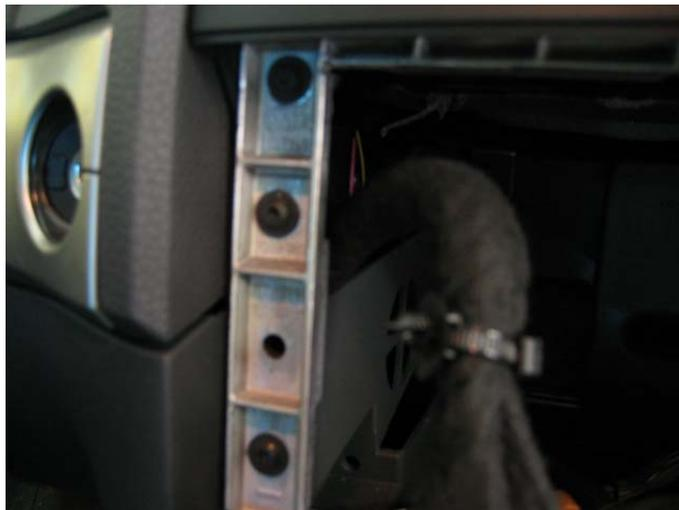
5. Gently pull bottom of bracket out by pulling from behind hazard and seat heater controls. Complete metal bracket will slide out from under vents.
