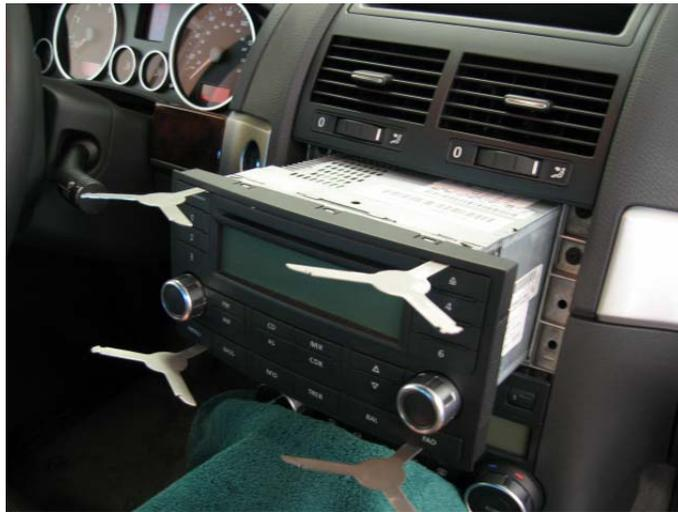
2. Remove 4 radio tools by pulling outward firmly.
