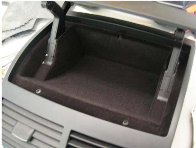
14. Reinstall assembly into dash by firmly pushing it back into place, just as you pulled it out. It will pop into place and be firmly seated when correctly inserted.
