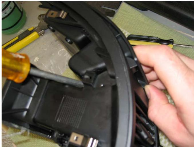
11. Remove old assembly and insert new Dash Storage Bin & Cover. Rear of bin will catch on vents and hold it in place.
