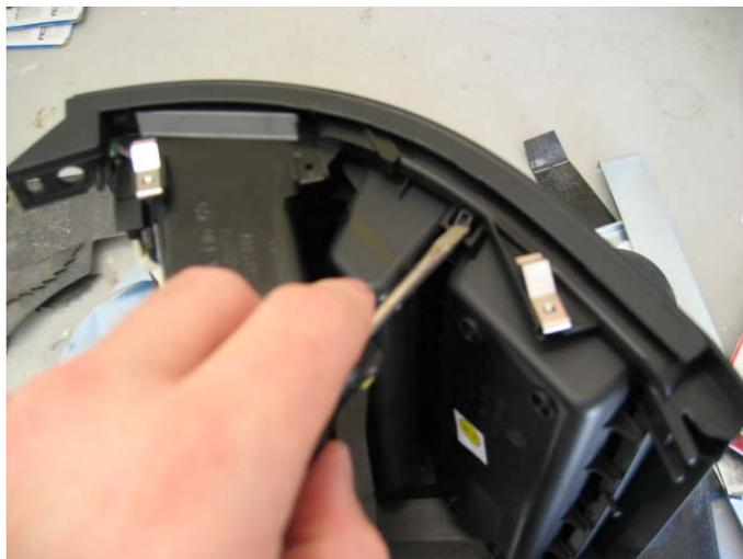
10. Use a longer screwdriver inserted between vents and old storage bin to release 4 tabs and allow old bin to completely release up and out of assembly.
