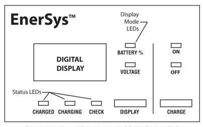
OMAX-12A-1B and OMAX-25A-1B CONTROL PANELS
