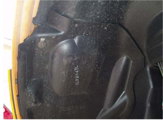
Undo the top screw first, then the bottom two. Take the screws out completely.
