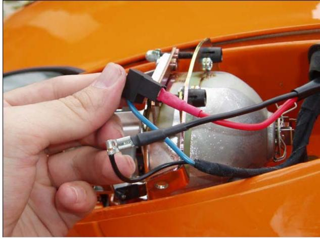
You may have to pinch down the end of the negative female connector, it was too 'loose' for the new male to fit into!!
