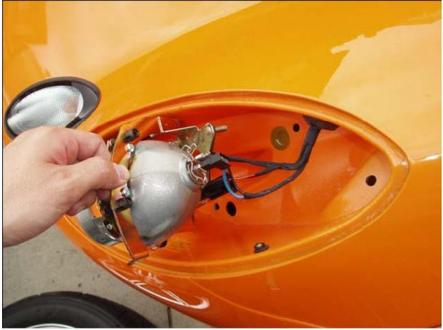
These two connectors shown here will be detached from the OEM bulb and be used to plug into the power-in side of the ballast assembly.
