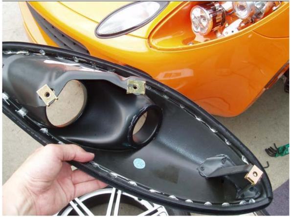
Now back underneath. Take off the nuts that hold the lamp assembly to the clam.
