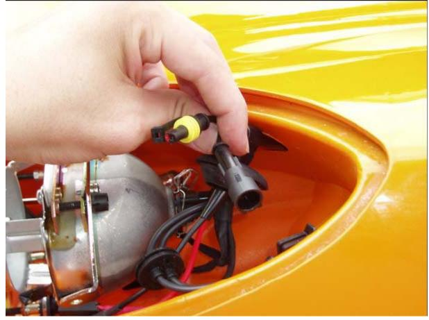
Shove them through the rubber washer. You may need two sets of hands to do this, one set: holding the rubber washer and with a screw driver, stretching the hole open; the other set pushes the connectors through one at a time. Now put the rubber washer back in place.
