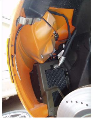
A close-up of the area you will be working on. The three nuts hold the lamp assembly to the clam. The three alen-bolts hold the lens cover to the clam.
