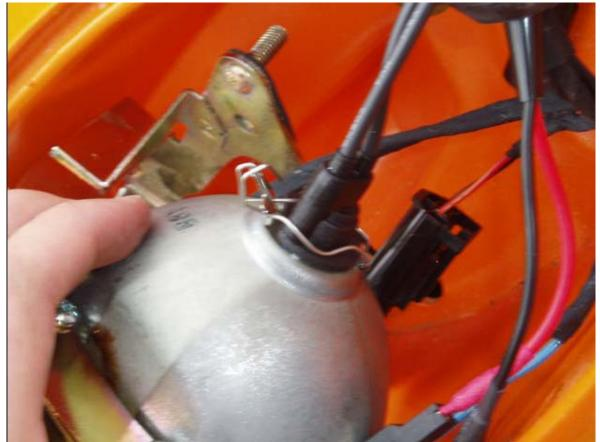
Now feed the power-out end of the ballast into the light area.
