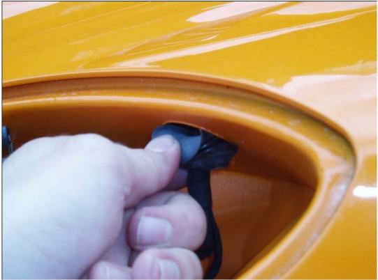
Now assemble the wires that connect to the ballast. The two male ends (3-oclock in the picture below) are going to plug into the female ends that originally plugged into the back of the OEM light bulb (shown prior). The middle connector/adapter gives us some length. The ballast is not shown here (sorry), but just off to the right. The plug assemblies are designed to only allow you to construct this in one manner.
