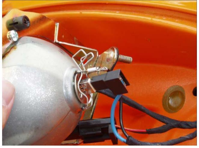
Loosen up the rubber pass-through part.
