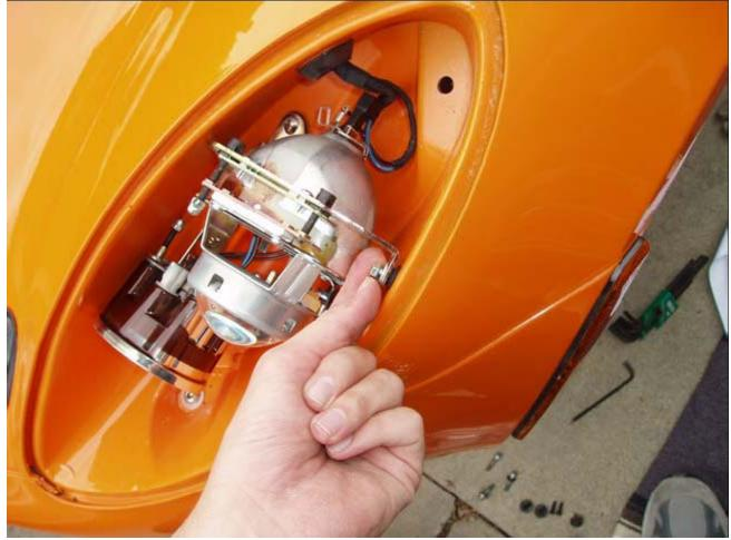
This is what that bolt was screwed into. Don't loose this, because it is prone to just fall out and roll off into the grass. You can leave it in place or add it to your parts list.
