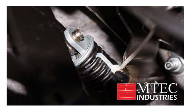
Wedge the screwdriver between the rod assembly and clutch pedal assembly to reinstall pin.
