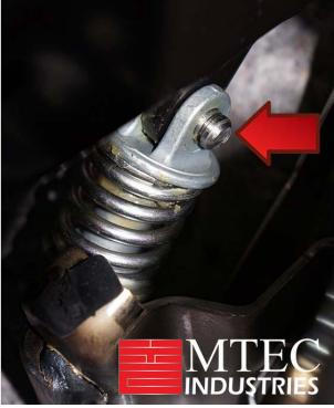
Once pin is removed place the screw driver in the same location. While pressing down with the screw driver Press the clutch pedal at the same time to remove the rod assembly and spring from the pedal assembly.
