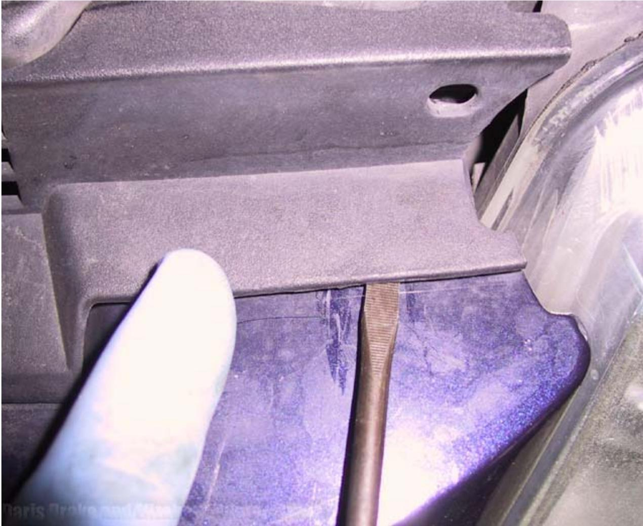
2: Remove the bumper skin. First pop the two side marker bulbs out of the housings. There are 4 torx screws in each wheel well (turn the wheels to access them or use a torx socket), five under the grille, and one behind each of the lower side grilles. Once they are off the skin will be free. It is very light and does not pose a danger: remove it and place in a safe location.
