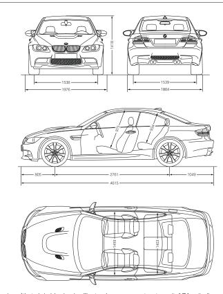
All dimensions of the technical drawings in millimetres. Luggage compartment capacity (VDA method): 430 litres.
