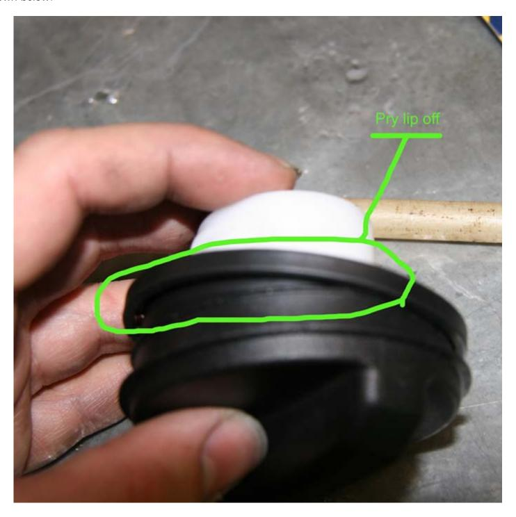
Once the ring is removed, you can begin removing the center threaded portion of the cap:
