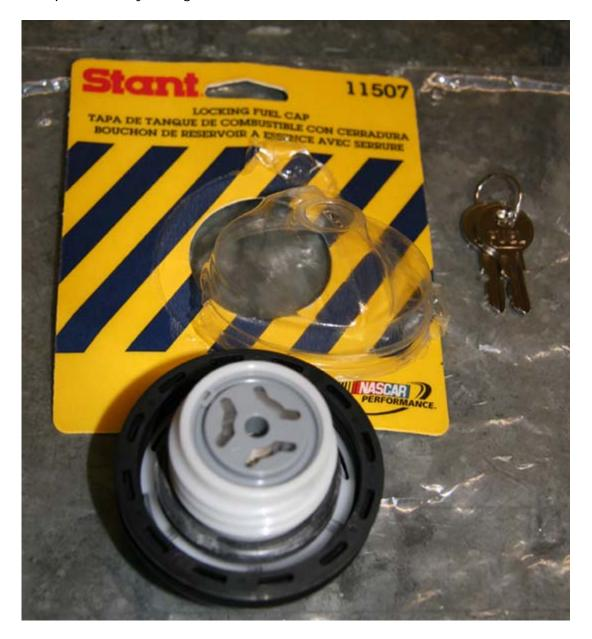
There is a plastic ring on the bottom of the black part of the cap. Using a small screwdriver, pry this off, as shown below:
