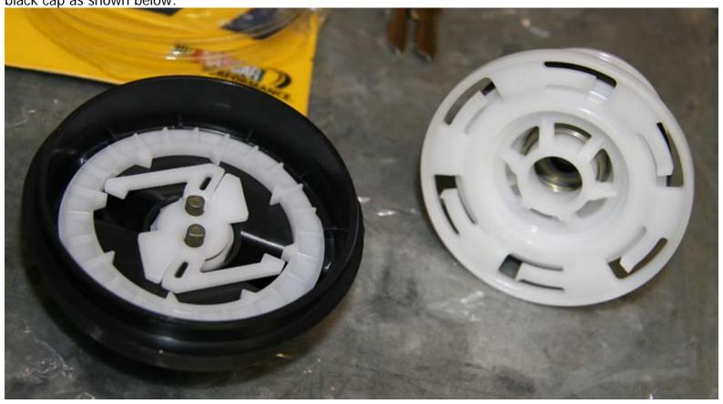
Re install the Stant ring, locking the Elise's fuel spout fitting onto the Stant locking gas cap.
