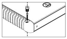
The standard method of mounting requires removal of the four corner caps with the 3/16-inch hex wrench included with your amplifier. Using appropriate mounting screws (not included), secure the amplifier in all four corners and replace the corner caps.
