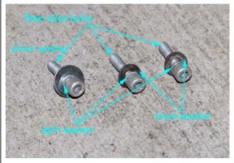
Once the three allen bolts are removed, you can remove the headlight cover. To do this, you pry against the rubber gasket on the headlight cover on the outside of the car towards the front of the car. Once the cover slides forward an inch or two, you can guide it past the low beam projector and the high beam reflector.
