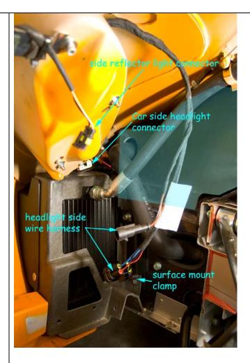
For the passenger side, I was only able to attach with the wires exiting towards the front of the car.
