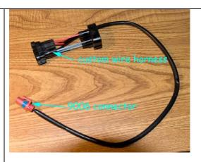
You can transfer the anchor point from the factory harness to the custom wire harness because it gets crowded near the turn signal by the connector. Plug the car side connector into the custom harness and the custom harness to the headlight harness.
