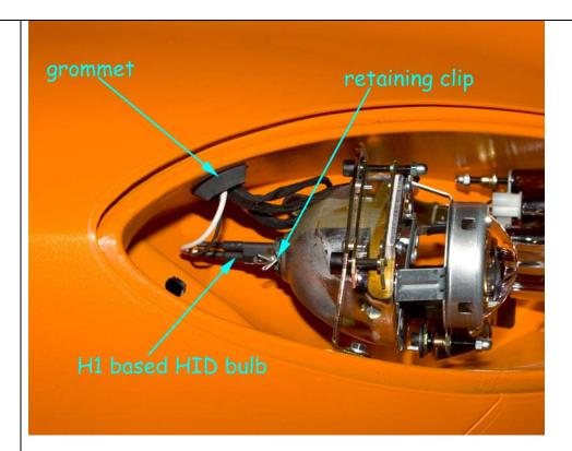
Now pass the remaining connectors through the opening. Reconnect the high beam and the DRL (for lack of a better term) connector. The stock lowbeam connector can be left dangling as it will not be powered (the custom wire harness does not feed power to the old lead). You can, however, attach the grounding spade to keep it out of the way.
