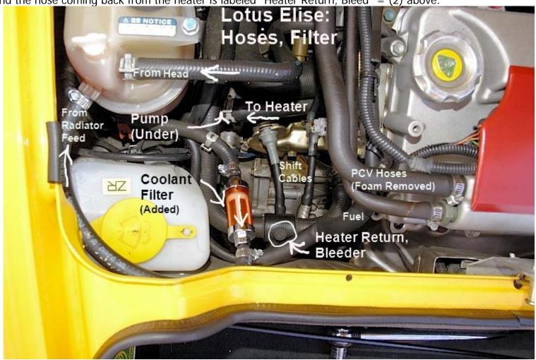
Here is the radiator bleed. Access it from the RF wheel well with the liner removed...or from above. Remove access panel and RH grill half. Use skinny or offset screwdriver, then turn by hand if you fit. The radiator bleed
