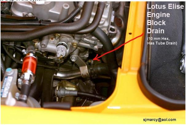
Here is a blown Hass Turbo Elise block ready to come out of the car...good view of the block drain...it lives under the #4 exhaust port...to drain the block you use a 10 mm wrench on the RHS bolt and the engine drains out the tube on the left:
