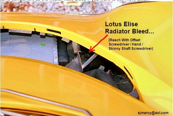
Accessing the radiator bleed screw...use a skinny screwdriver...this is 99 and 44/100ths % easier than the Lotus procedure. They have you lift or jack up the car...remove the RF wheel and wheel liner for access. Again: Instead just remove the service panel (one screw..use 3 mm allen wrench from the tool kit) and the RH half of the black grill (two allen screws, same tool). Then access the bleed with a skinny screwdriver. Same oringed plastic bleed screw as the bleed for the heater hose.
