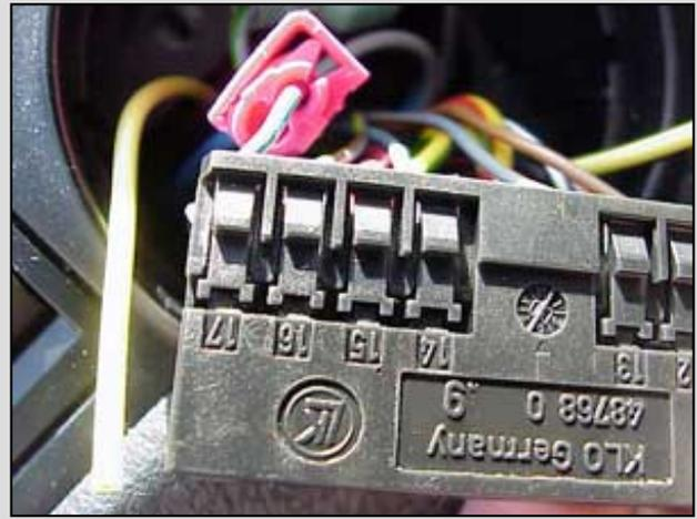
Locate pin 17 on the harness connecting to the light switch. Using the supplied Scotch-Lock, tap into the GRAY wire with BLUE stripe coming from the #17 location. Re-Install the headlight, wait till dark, turn on the lights and feel the love.
