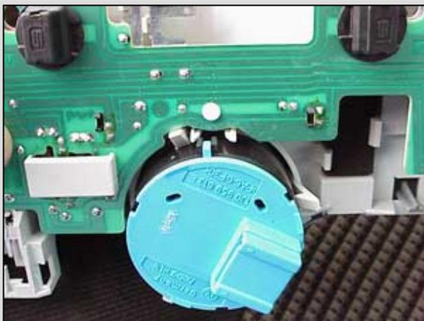
Install the old knob into the new W8 light panel. Note the orientation of the black/blue/black tab on the switch; It should face the bulb sockets in the panel. Before seating the switch, flip the panel over and check that the knob rotates correctly with the markings on the panel.
