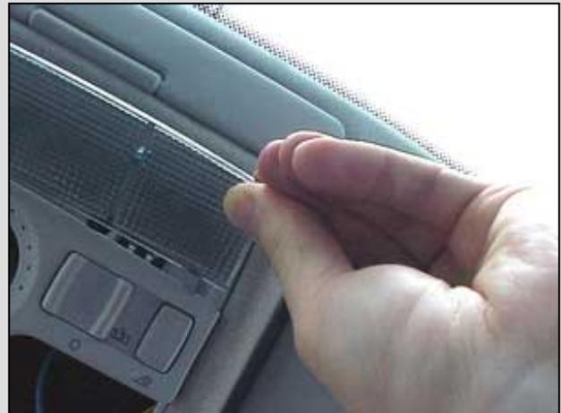
The lens will simply flip down and pull out.
