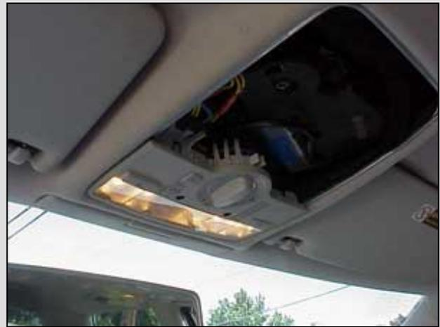
Tipping the drivers side up first, then let the passenger side snap into place. Push the module towards the front of the car. (Note the wire harness in this picture was a prototype)
