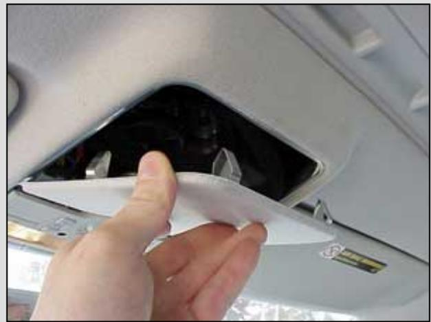
Remove the cover from the sunroof motor compartment. This is held in with just simple spring clips. Pry down with your thumb, using screw driver may help here.
