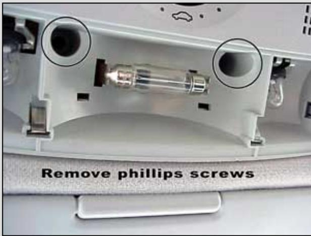
Remove the two phillips screws from behind the lens cover.
