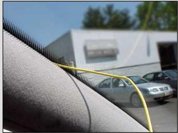
Run the long wire from the ECS thru the headliner, thru to the windshield or straight over to the A-pillar. You will need to run this wire down to the back of the headlight switch.
