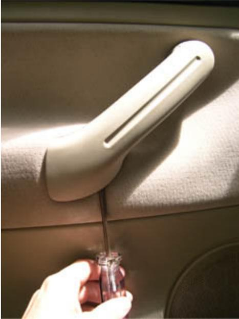
11. Once one end of the outer handle piece is pried out slightly, move to the other end and pry that out slightly, as shown below. Go back and forth between ends until the handle has been pried out approx. 1/8". Once it is this far out, you should be able to pull it off the rest of the way with your hands.
