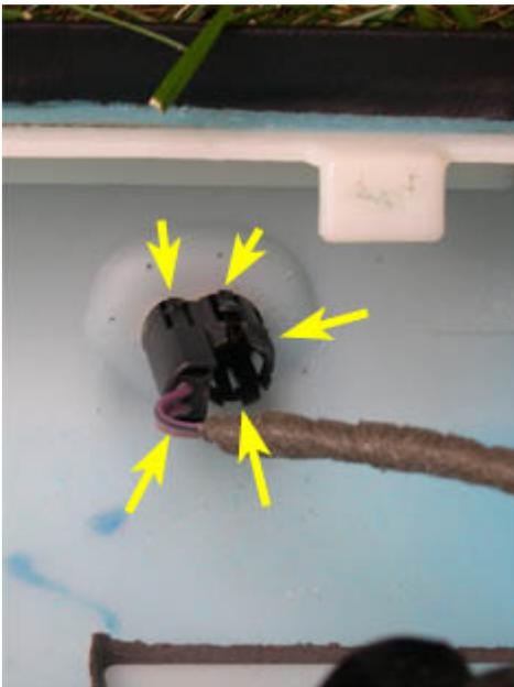
31. To remove the door light, push in on the two tabs indicated by the arrows in the picture below and slide the light out of the door panel.
