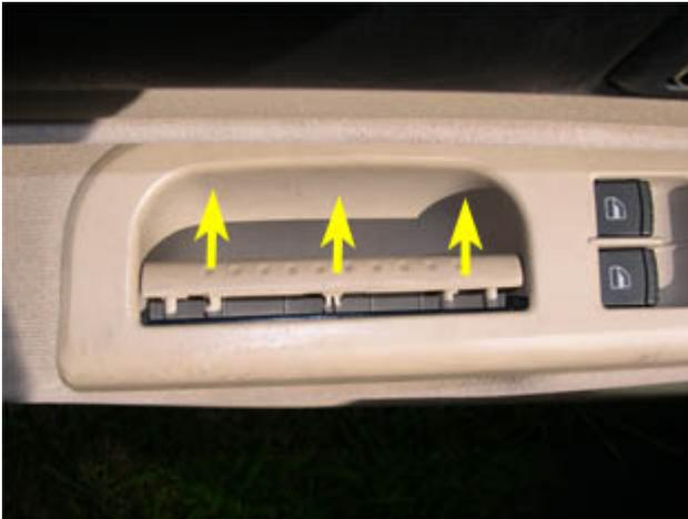
5. To take the main handle piece off of the driver's door panel, pull the rear of the handle upwards to unclip it, as shown below. Do the same at the front edge of the handle.
