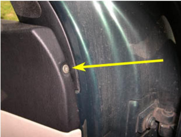
16. Starting at the bottom of the door, pull the door panel away from the door, as shown below. There are six snaps securing the panel to the door, three near the front edge of the panel and three near the rear edge of the panel. The approximate location of the two lowermost snaps on the rear edge are indicated by the red spots. After unsnapping the six snaps, the door panel should still be attached to the top of the door near the bottom of the window.
