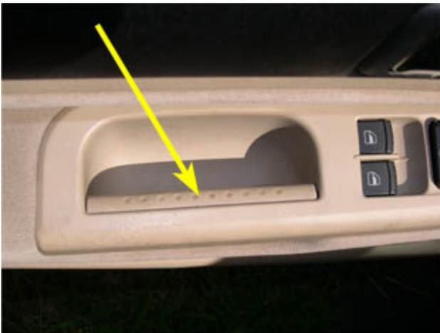
3. Insert a screwdriver or other strong, thin tool into the crack between the inner and outer pieces, as shown below, and carefully spread them apart. Be careful not to harm the soft-touch coating on the handle pieces - you may want to protect the tool with a thin rag. Although a screwdriver is shown in the picture, I actually prefer a tool with a wider blade, such as a putty or spackling knife - it has always been easier for me to get the handles off with one of these.
