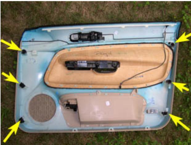
18. Starting with the top, rear corner, pull the door panel up and out of the window seal, as shown below.
