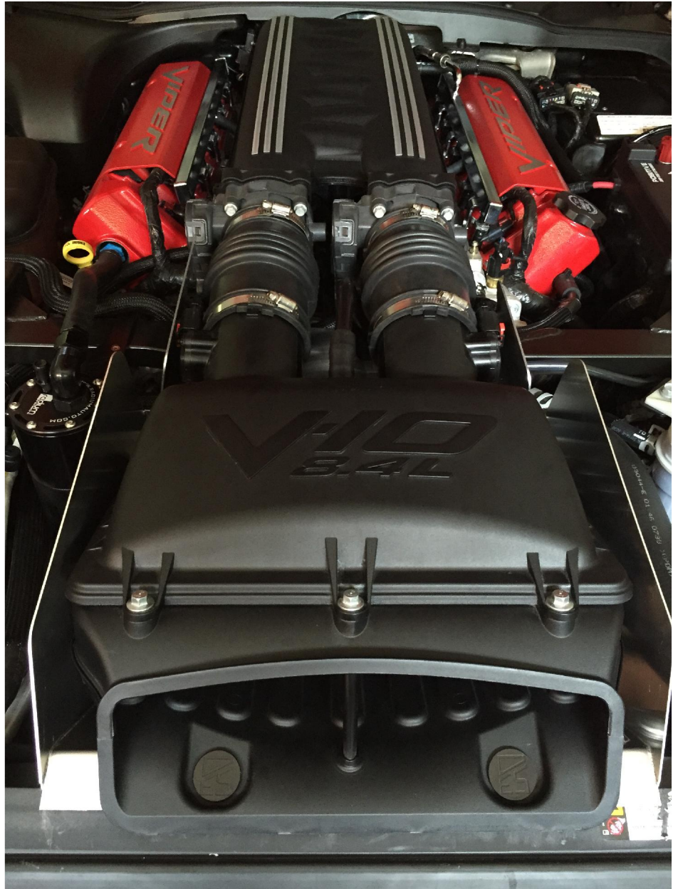
Heat shield and air cleaner assembly installed (Gen IV, Uncoated Shield)
