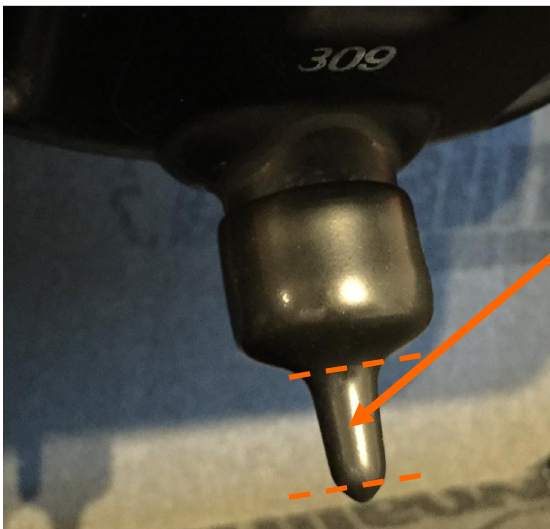
DSE Alternative to OEM P/N 05038304AA (Cut to allow water drainage from airbox)
