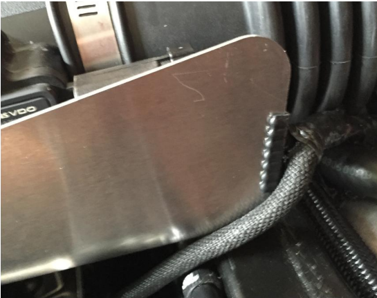
Anti-abrasion edging installed (Gen IV Only)
