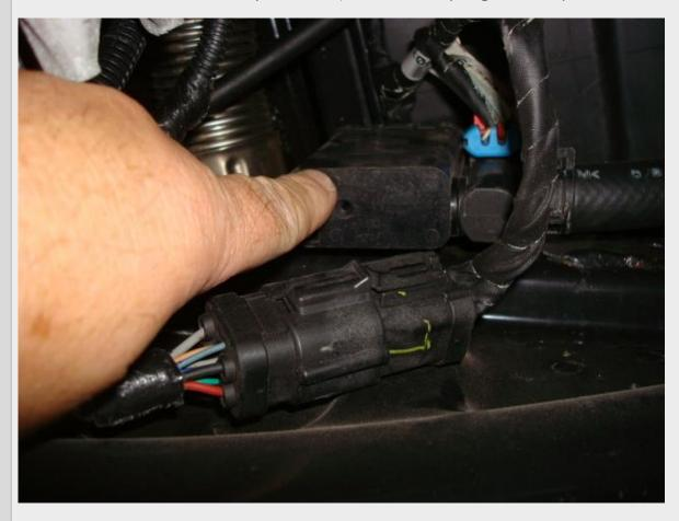
Remove the Vent Hose (it runs to your emissions canister) using a pair of pliers. You can rotate the clamp if needed to access the dog ears to open the clamp.
