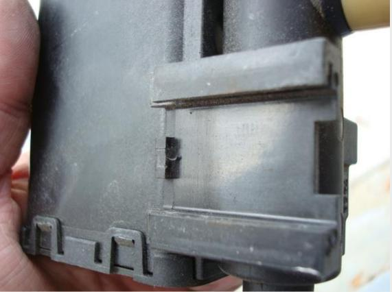
Put the new Vent Solenoid Assy back on by placing it on the bracket and slide it towards the front of the car. You will hear it click in place. Plug the power plug back in and reconnect the hose.
