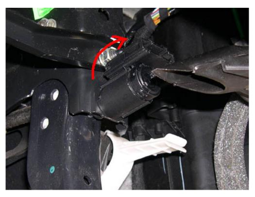
7. Connect the wiring harness to the switch, as shown in the picture below. The switch has been installed correctly and should now work fine.
