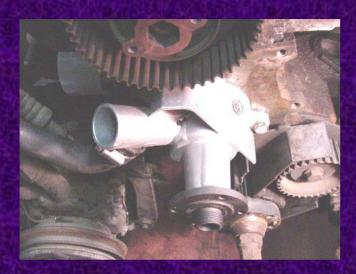
Install the new water pump using a NEW gasket, smeared lightly on both sides with Permatex gasket stuff. Mount with the 3 bolts. Torque properly.
