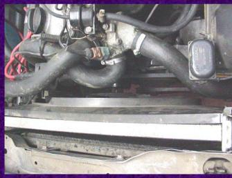
Replace the shroud first, then the radiator. Reconnect all electrical connections to the right top side of the radiator.
