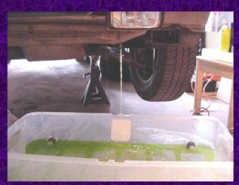
Drain the coolant from the system, and make sure you also drain the engine block by unscrewing the 19mm drain plug by the exhaust manifold.
