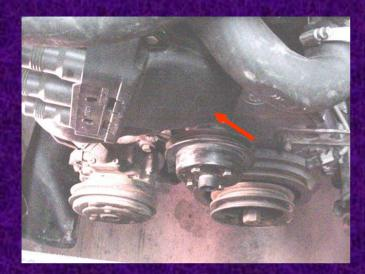
Reinstall distributor shield, rotor and cap. Now, put the drive belts, the alternator belt and the A/C belts back on, and tension all belts properly.
