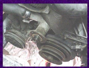
Remove the fan belts by loosening the star adjusters, slackening the alternator and steering pumps off, and removing the belts. Remove the spark plugs and rotate the engine to TDC... Leave it there and mark positions with paint!
