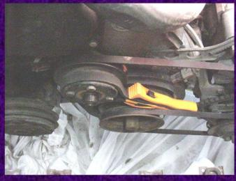
I also used the strap wrench to hold the water pump pulley while I removed its 4 retaining bolts.
