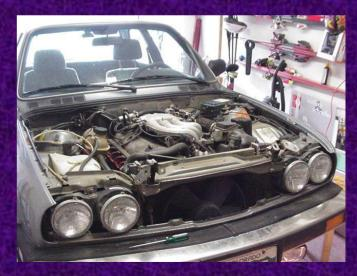
Remove the radiator by unhooking the shroud, hanging it on the fan, disconnect the top hoses and the bottom hose, and undo the two bolts and remove it
