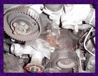
Remove the tensioner gently, making sure that the spring and adjustment pin don't fly out!
