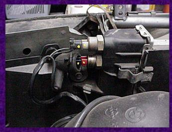
Mark everything well. Here I've marked the proper wiring attachments for the radiator electronics.
