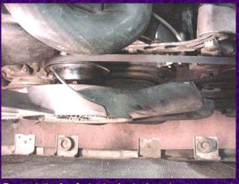
Reattach the fan & clutch. Again, I used a strap wrench to hold the pulley steady and the Channel-Locks to tighten the fan nut to the water pump shaft. Remember, it goes on COUNTER-CLOCKWISE..
