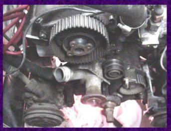
Remove the two upper bolts from the top timing belt cover, the alternator bracket, the top cover, then the lower cover bolt and cover. Loosen the top bolt on the tensioner, push it left, retighten. Snake out the belt.
