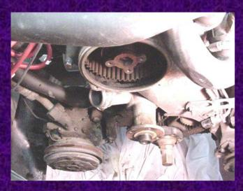
Remove the 6 hex bolts from the crankshaft pulley, and remove it and the vibration damper behind it from the car. The vibration damper is indexed and has no separate bolts.
