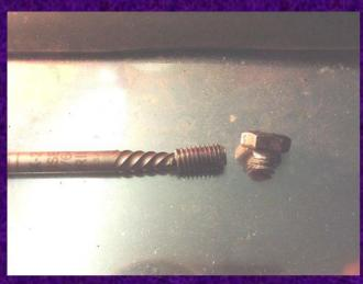
This is where I ran into trouble. I over-tightened the lower timing cover bolt and it sheared off. I was able to drill out the center of the broken bolt an removed it with an extractor.
