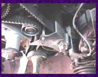
After getting the sheared bolt squared away, I mounted the lower timing belt cover.
