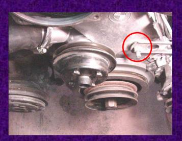
Install the water pump pulley and the main crankshaft vibration damper and pulley. Torque bolts to specs. Notice the alternator bracket correctly attached unlike last picture.
