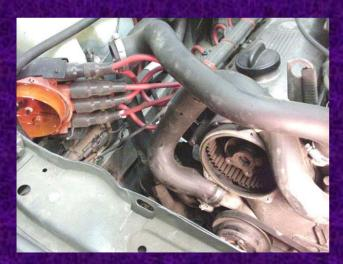
Remove the distributor cap and rotor, pushing the cap aside, with the wires still connected..
