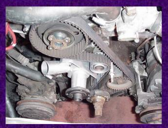
Install the belt. Start at the bottom, around the lower gear, around the tensioner and up to the top timing gear. It'll be a tight fit and you have to gently ease it on. Unscrew the bolt holding the tensioner, and let it spring into action. Tighten tensioner bolts
