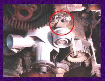
Install the tensioner, making sure the adjustment pin seats in the receptacle on the water pump and the pin is through the tensioner bracket. Push it ALL the way to the left and tighten down.
