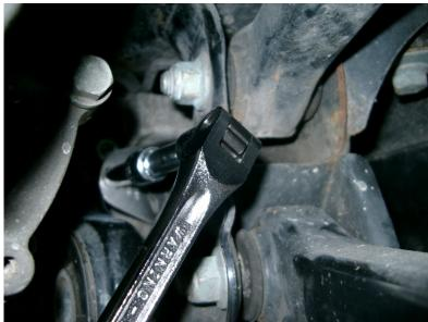
5. Push the wrench forward to loosen filter. Once loose remove it by hand.
