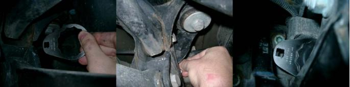
4. Install the socket wrench and extension bar into the H-Wrench as shown.
