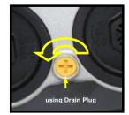
**D.** With the housing drained, the two fuel filters may now be removed. Ensure the catch basin is still in place. Loosen and remove the first housing cap. To do this, use appropriate socket with a 3/8" ratchet and turn the housing cap counterclockwise.
