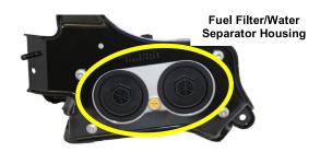
C. Drain fuel filter/water separator housing. To control spillage, place a catch basin underneath the fuel filter/water separator housing. Using a large Phillips screwdriver, loosen the housing drain plug (turning counterclockwise) to empty the housing of any water and fuel. Once drained, tighten the drain plug. Be careful not to overtighten the plug. Wipe up any spilled fuel.
