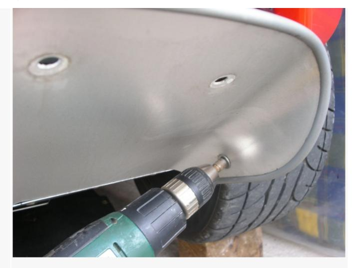
6. Now the diffuser is held by the 2 large dome-headed Allen screws in the centre of the panel. Lie under the panel, supporting it with your shoulder and remove the screws using the 5mm Allen key (13mm bolts on '06 Model):
