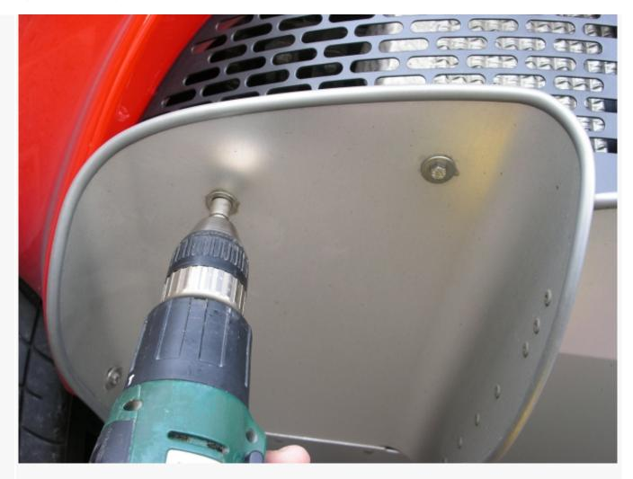
5. Look at the turned down edge of the tunnels, immediately behind each rear wheel. Remove the 2 dome-headed screws and nuts (one set each side) using the 4mm Allen key and a 10mm socket on the nuts (8mm bolts on '06 Model):
