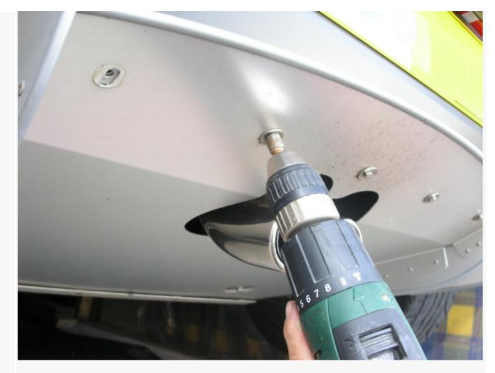
4. Remove the setscrews at the rear edge, one 2 on '06 Model in either "tunnel" of the diffuser:
