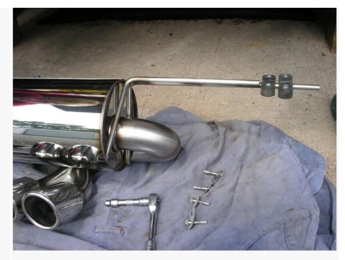
16. Spray some WD40 into the LHS exhaust mounts and on the Cat pipe.
