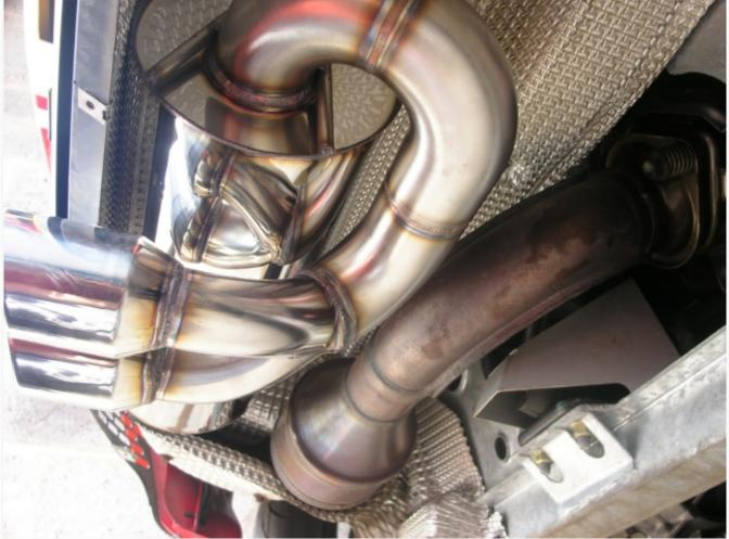
(In the above picture, notice how the silencer is actually touching the heat-shield at the rear of the car. That is not by design of course and I'm not sure whether it's as a result of other '06 Model changes, but I eased the heat-shield away from the silencer and no vibration / rattles are present. Will need to monitor that situation however)
