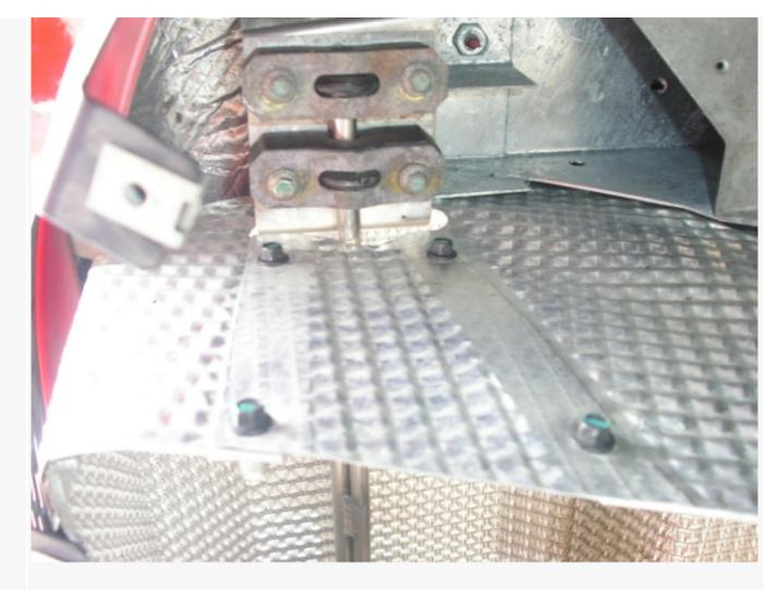
19. I recommend swinging the silencer tailpipes as high as you can up to the number plate panel. This increases the clearance at the Y-piece as it comes down through the diffuser. There should be a 10mm gap between Tailpipe and the number plate panel. Look up through the Tailpipes and centre the threaded hole in the number plate panel in the gap between the pipes by puling/pushing on the silencer.
