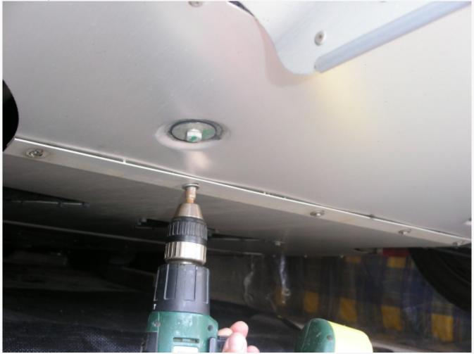
3. Go to the rear edge of the diffuser, below the number plate and remove the 3 (5 on '06 Model) setscrews there with the 8mm socket:
