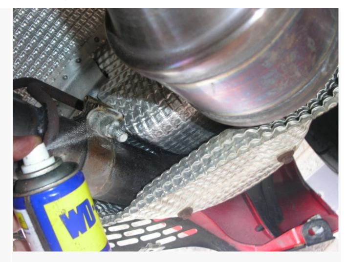
9. Loosen the exhaust clamp, using a 13mm socket. It's welded to the pipe so won't come off – just make sure it's well loosened.
