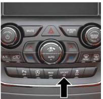
Your vehicle is equipped with a Sport Mode feature. This mode is a configuration set up for typical enthusiast driving. The engine, transmission, and steering systems are all set to their SPORT settings. Sport Mode will provide improved throttle response and modified shifting for an enhanced driving experience, as well the greatest amount of steering
