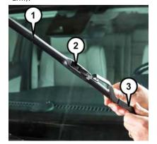
Wiper Blade Removed From Wiper Arm
