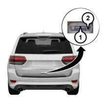
Electronic Liftgate Release/Liftgate Passive Entry Location
