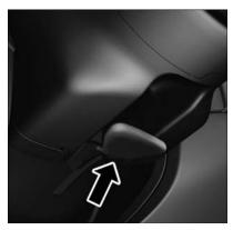
Manual Tilt/Telescoping Steering Column
