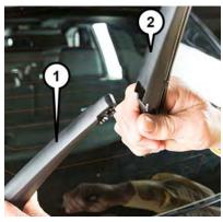
Wiper Blade Removed From Wiper Arm
