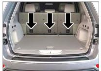
Top Tether Strap Anchorage (Located On Seatback)
