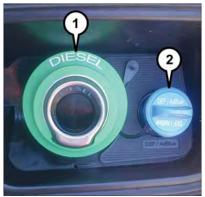
Fuel and Diesel Exhaust Fluid Fill Location
